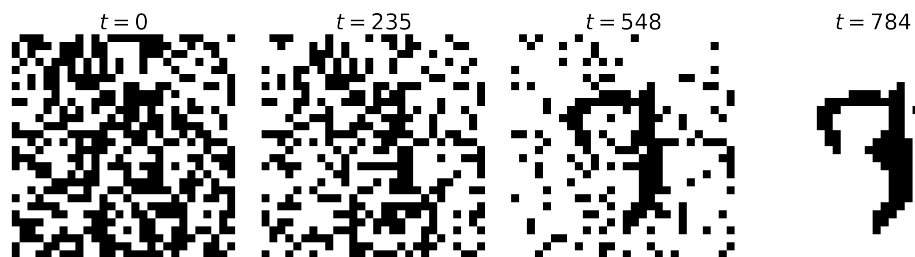
Figure 2.7 – A discrete Hopfield network (DHN) converging to a spurious attractor when initialized from a random state. In McCallum’s pseudorehearsal protocol, many of the recovered states correspond to this kind of spurious attractor.
